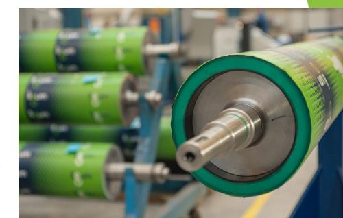
SMOOTH COATING sleeves for varnishing or with "OPTI/ RILI" cuts; 20-50' ShA
